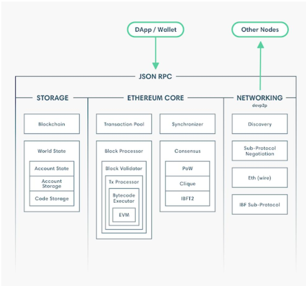
The JSON RPC layers and below in the above diagram are a part of the existing Besu implementation. It has already reached the maturity level of being compatible and working with the Ethereum mainnet, and has been deployed in live environments.
