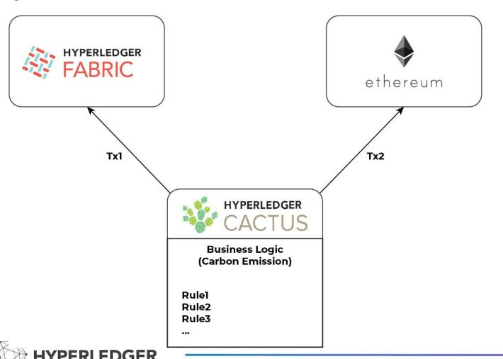
**Tx1** - converting the energy into emissions
