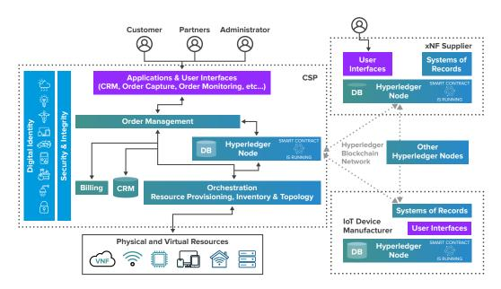
FIGURE 4: REFERENCE ARCHITECTURE FOR END-TO-END LCM FOR IOT USING HYPERLEDGER
